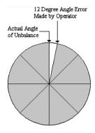
For small angular errors the percentage error can be calculated by multiplying the sine of the error angle (x) in degrees by 100 to get percentage.
